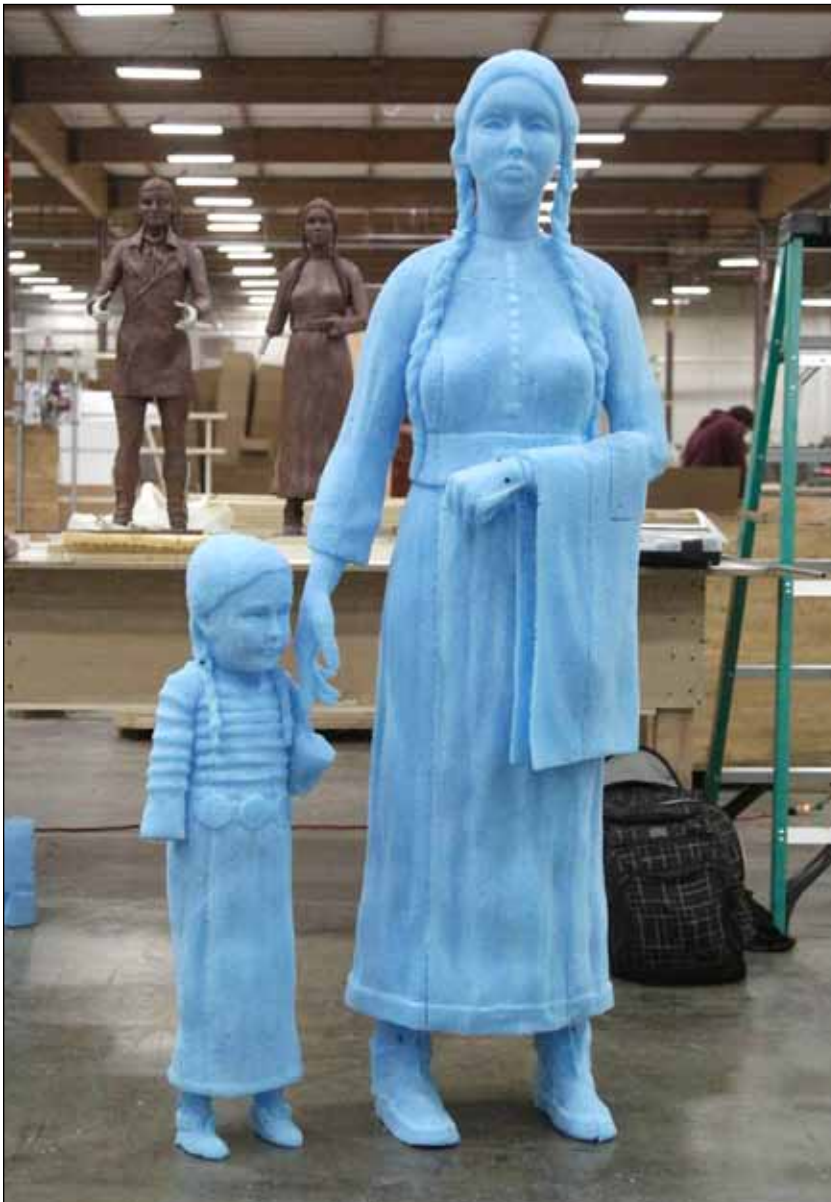
Foam models of Robert Dickson’s wife Ista Totowin and their daughter Helen Dickson that are part of the bronze casting process. (Photo by Jean-Sébastien Gauthier)
